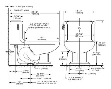
THIS TOILET IS DESIGNED TO ROUGH-IN AT A MINIMUM DIMENSION OF 12" (305MM) FROM FINISHED WALL TO C/L OF OUTLET.
